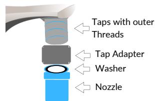
For Taps with M22(Outer) Threads, Place the adapter & Washer above the Nozzle and insert into the Tap and Fix it well.
