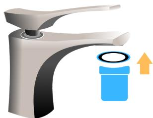
For Taps with F24(Inner) Threads, Place the Washer above the Nozzle and insert into the Tap.
