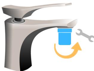
Fix the Spanner and Rotate Clockwise. Tight enough to fix it firmly.
