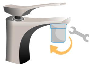
Use the Spanner or Wrench, Remove existing nozzle or aerator by turning Anti-clockwise direction. Remove the Aerators along with Washers.
